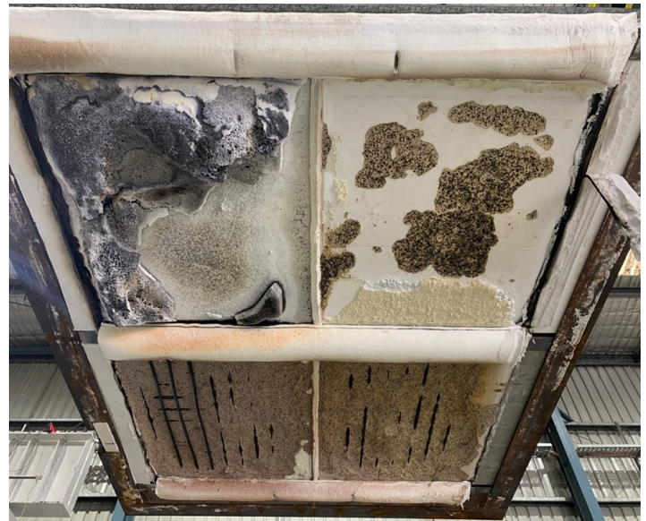
Four flat panels after fire testing [SOURCE: SUPPLIED]
